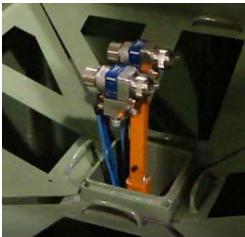
Quick Change Inside Spray Gun on Linear Actuator *Shown with dual gun option
