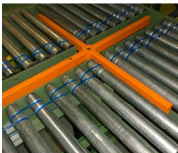
Infeed Conveyor with Pneumatic Lift Cross
