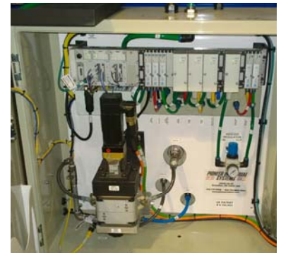
Patented Servo Controlled Precision Fluid Delivery Panel US PATENT 9,192,953
