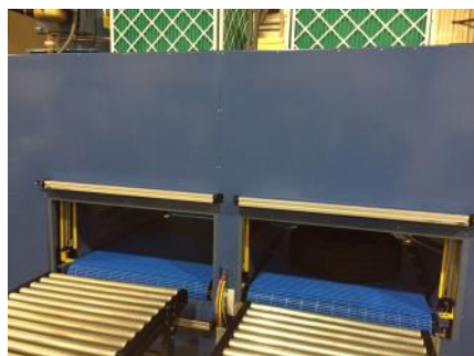
Dual Conveyor WWS2-1000o 360 *tire per hour with Fanuc LrMate Robot
