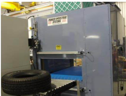
Single Conveyor WWS-1000o 240 *tire per hour with Fanuc LrMate Robot
