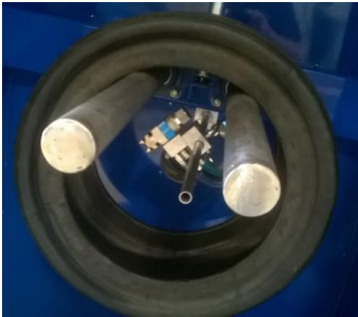
Quick change spray gun & manually adjustable positioning of the spray gun. Knurled rollers to provide grip.
