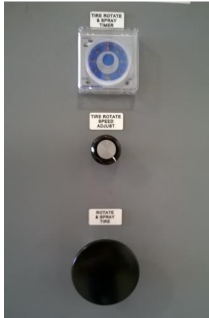
Adjustable timer to allow tire to get up to speed prior to painting. Potentiometer to adjust tire rotation speed. Push button starts & keeps the tire rotating. Tire stops when the button is released.
