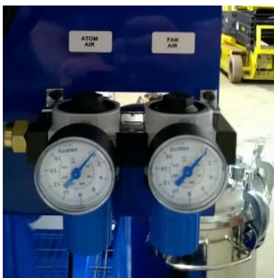
Manually adjustable regulators for Fan and Atom air pressures.
