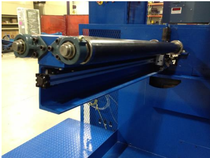
Quick change spray gun attached to linear actuator. Knurled rollers to provide grip to rotate the tire.
