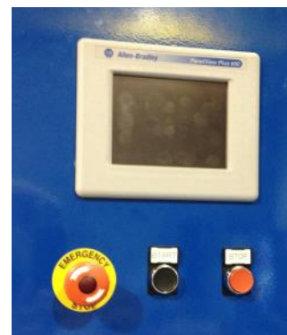
6" HMI, E-stop button, cycle start, & cycle stop buttons
