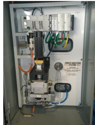
Servo Controlled Precision Fluid Delivery Panel US PATENT 9,192,953
