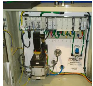
Optional Servo Controlled Precision Fluid Delivery Panel
